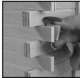
4. Now you will glue the  $\frac{3}{4}$ " squares or "log ends" onto the **backside** of each log that extends out past the interlock. Each  $\frac{3}{4}$ " square should be flush with the log you are gluing it to. This forces the side wall tight to the front wall and eliminates the need to actually glue the walls together.
