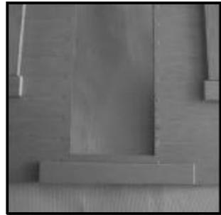
2. With the front wall face down, position and glue the first floor support under the front door opening. Keep it flush with the bottom edge of the wall and centered under the door opening.
